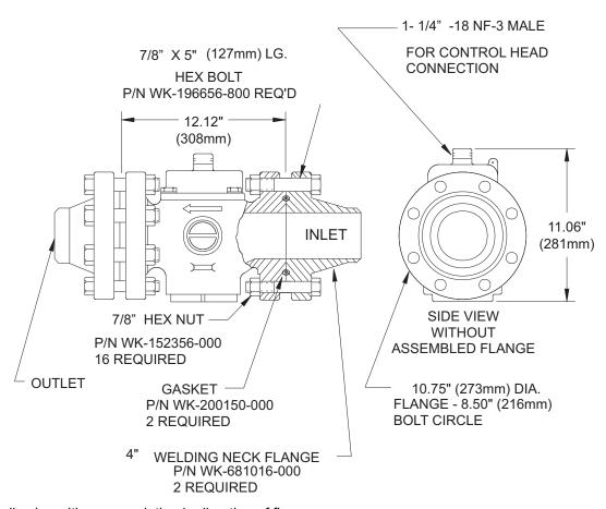
Note: Install valve with arrow pointing in direction of flow.
